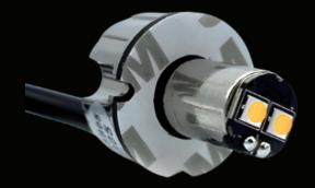
OUR HIDEAWAY COVERT LED RANGE MAY BE SUPER DISCREET, BUT WITH TWO LARGE LED CHIPS PER LIGHTHEAD THEY CERTAINLY GET NOTICED! THESE ARE E-MARKED, CE AND ECE EMC R10 APPROVED. A SMALL 13MM HOLE IS REQUIRED TO INSTALL THESE LIGHTS, THEY CAN BE EASY FITTED INTO VEHICLE HEADLIGHTS / REAR LIGHT CLUSTERS WITH THE PRE INSTALLED 3M SELF ADHESIVE GASKET (SCREW FITTING IS ALSO AN OPTION, SCREWS NOT PROVIDED).
