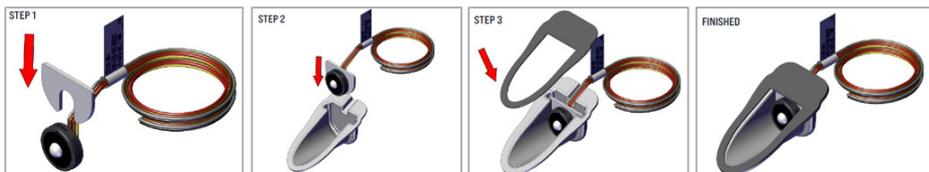
This installation guide demonstrates how to insert the Star-M1 in to the (SP\_DSXRPOD) window pod in 4 simple steps.
