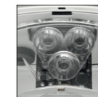
External LED Alley Lights
